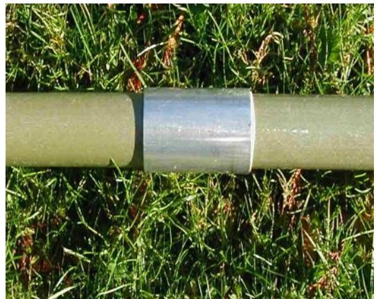
Fig 9: EST Extensions after sliding the top section over the bottom section
