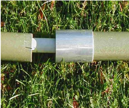
Fig 7: EST extensions with plastic diverter tube showing
